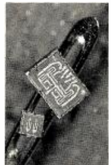
The transistor was invented at Bell Labs in 1947. Today, thousands of transistors can be made on one tiny integrated circuit chip.
